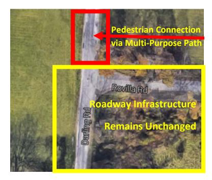
The portion of Darling Road west of the 90 degree bend will remain unchanged (see the area within the yellow below). The portion of Darling Road at the 90 degree bend will be modified to provide an access point and turnaround for emergency vehicles (see the area within the red below).
