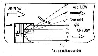
The high intensity germicidal light destroys or inactivates microorganisms. The nuclei of the cells of the microorganisms, due to photolitic processes caused by the CREON2000 system, are so changed that all cell division, and therefore reproduction of the organisms, can no longer take place. Because the CREON2000 kills the
