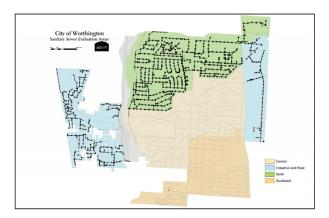
For the final phase of Worthington's SSES program required by the Ohio EPA, the City selected a 15-year program that included first investigating and secondly addressing capacity issues and excessive I/I in the sanitary sewer system. The SSES performed by EMH&T, identified sources and quantities of I/I entering the sanitary collection system, and feasible cost-effective actions to minimize excessive I/I entering the sewer system that caused or contributed to
