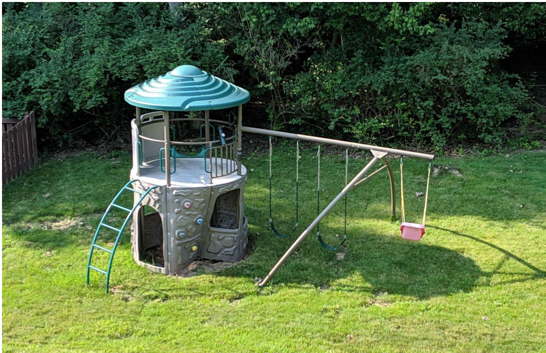
Fig. 7 | June 30, 2019 | A more direct look at the playset showing the damage to the support bar and damaged climbing wall. The support leg was dislodged and bent. Total repair costs exceeded $600.
