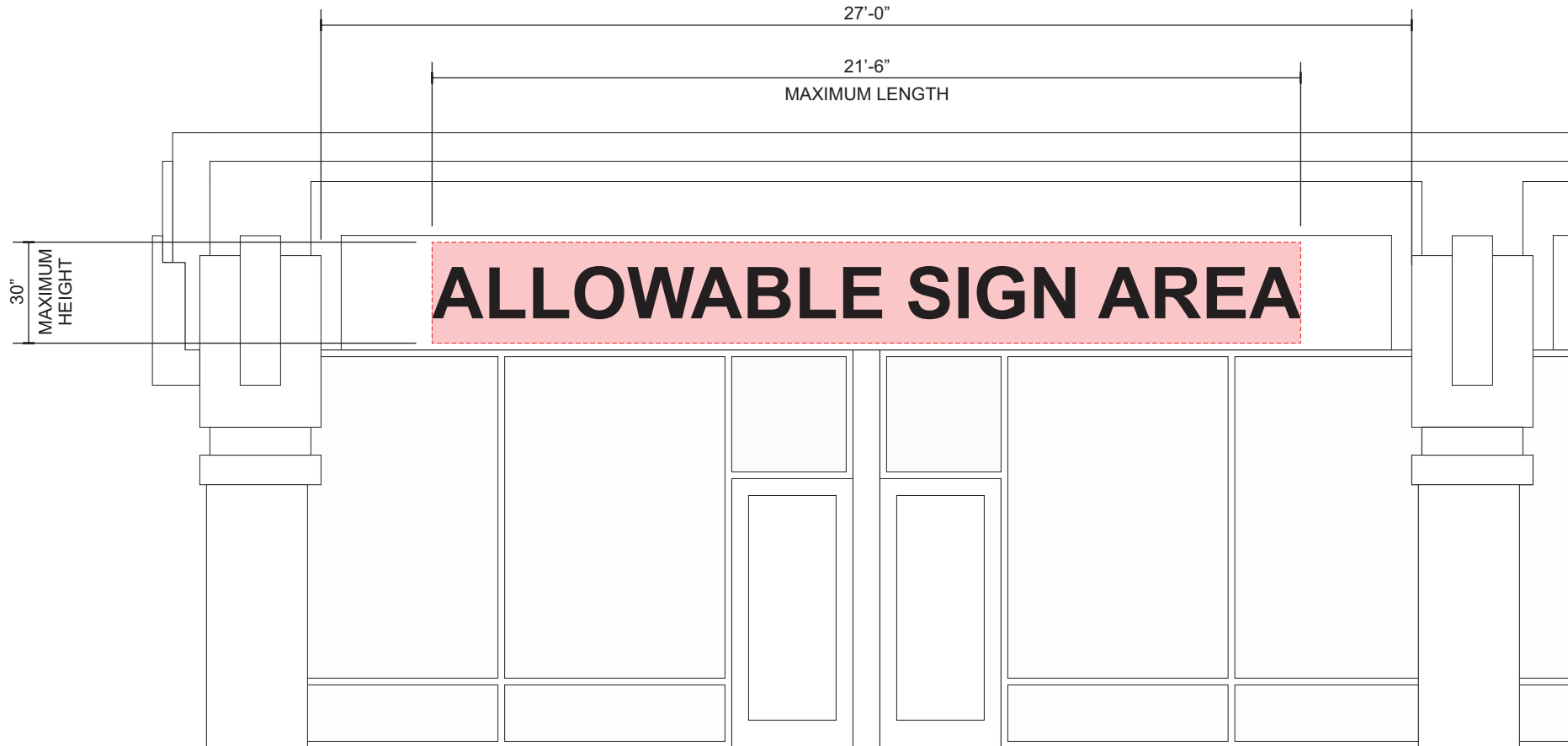
SCALE: 1/4" = 1' - WEST ELEVATION TENANT #1
