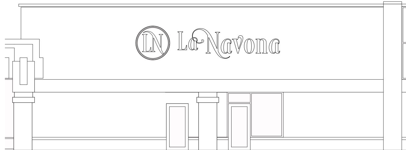
SCALE: 1/8" = 1' - EXAMPLE OF ANCHOR CHANNEL LETTERS
