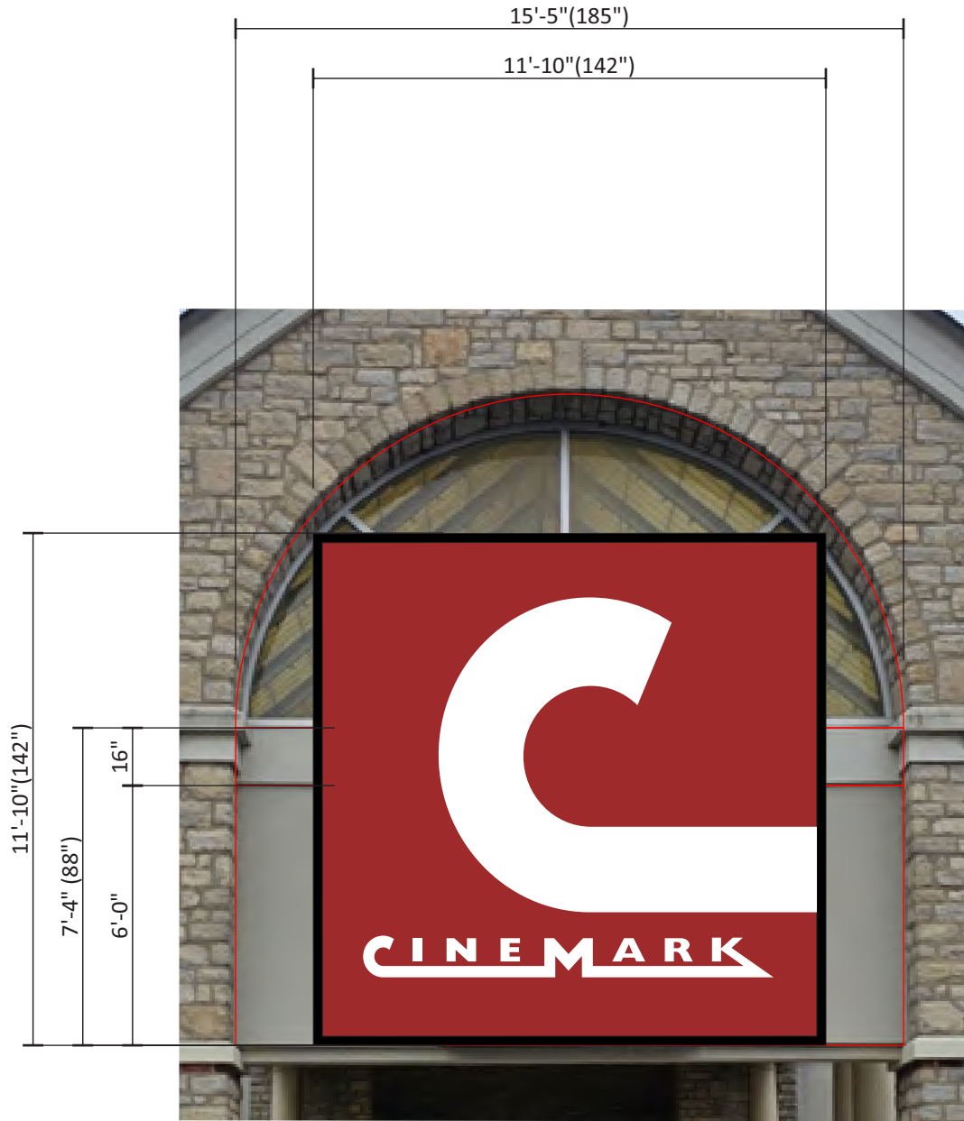
PROPOSED: PARTIAL BLDG. ELEVATION AT ENTRY
