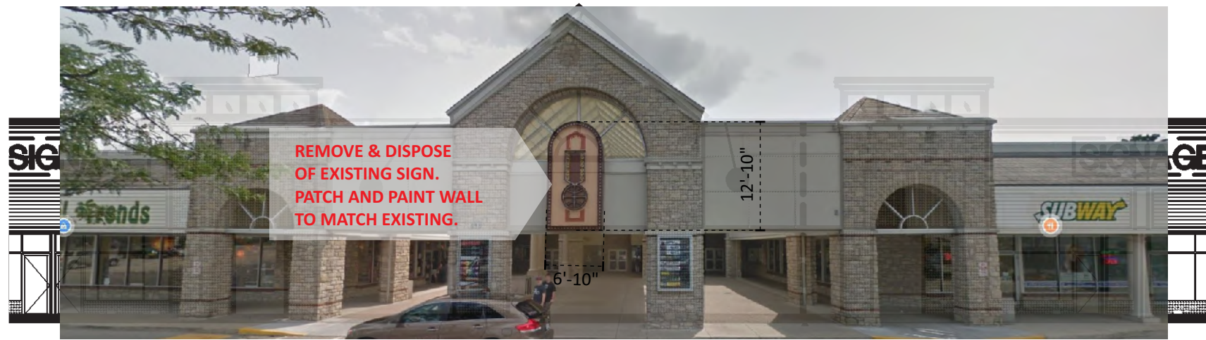
A EXISTING CONDITION: SIGN REMOVAL SCALE 1/16" = 1'-0" ONE (1) REQUIRED - REMOVE AND DISCARD
