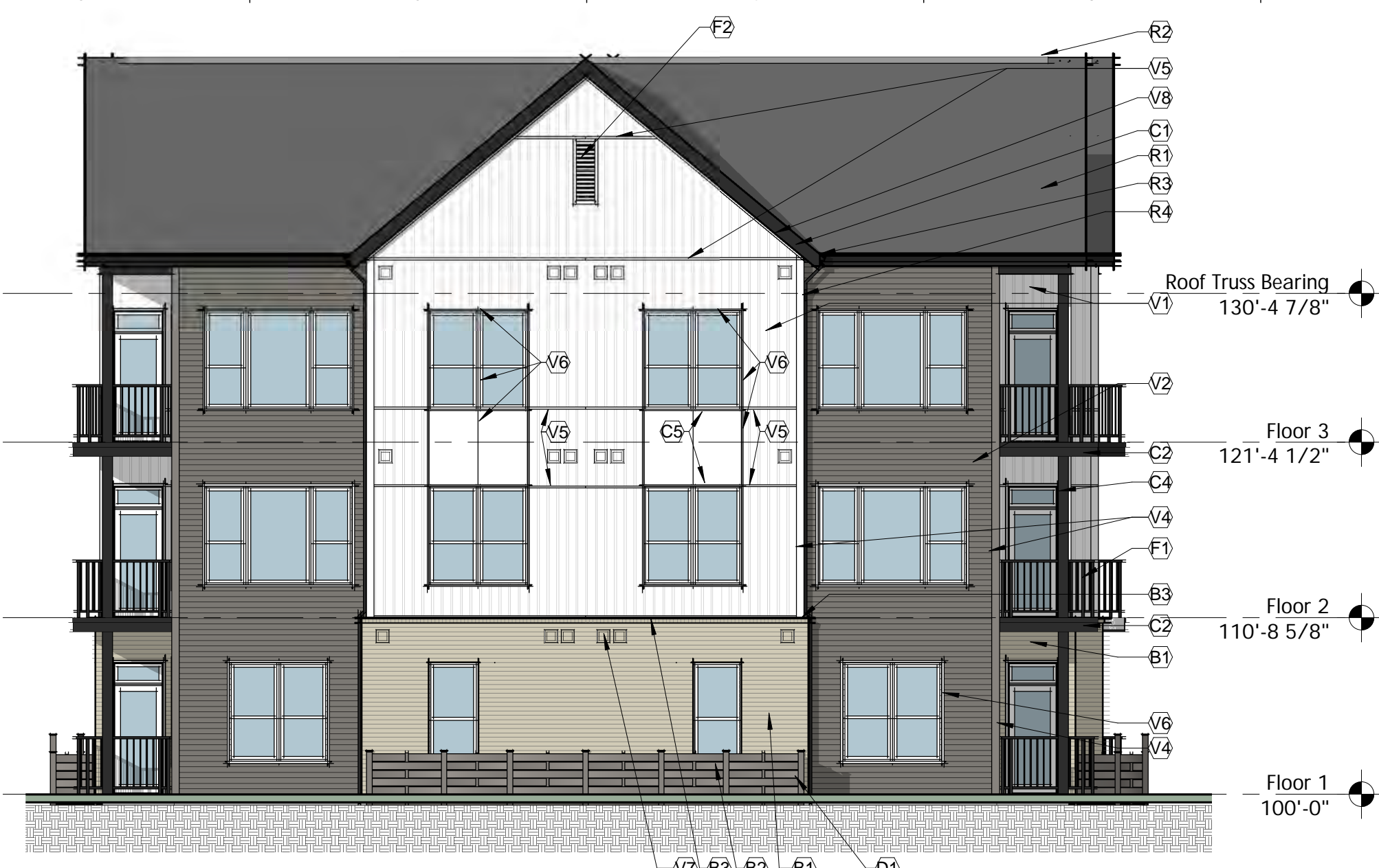
G4 Bldg. C Right Elevation 1/8" = 1'-0"
